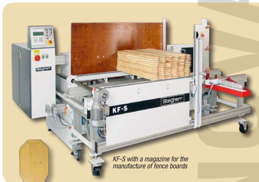
Milling of fence boards by means of a template
